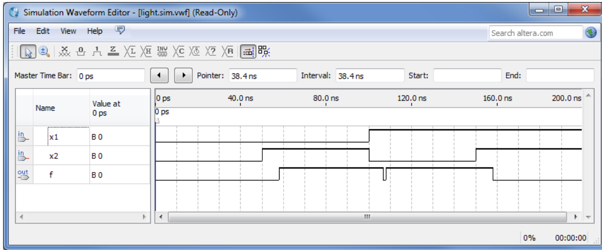
Figure 37. The result of timing simulation.
