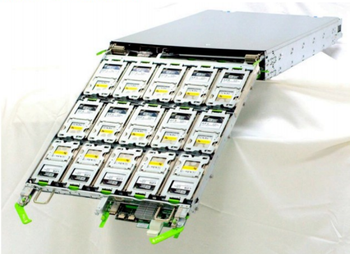
Figure 2 Open Vault Detail Showing the Hinged Disk Drive Tray
