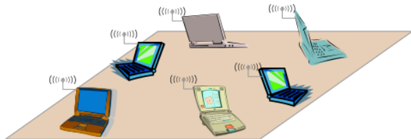
Figure: Simple example: laptops in a conference room – a single-hop ad-hoc network (all the networking nodes are in a direct communication range of each other node).
