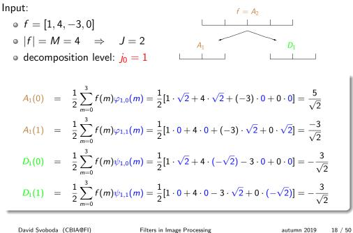
1D Discrete Wavelet Transform (DWT) Forward
