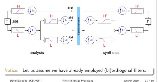
Subband Coding Signal Analysis and Synthesis
