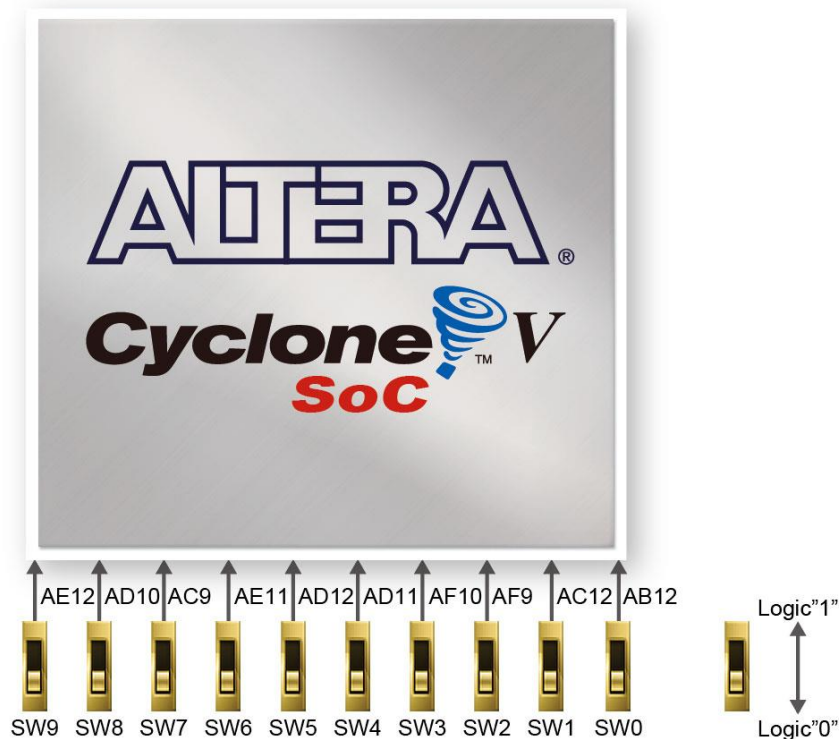
Figure 3-15 Connections between the slide switches and Cyclone V SoC FPGA
