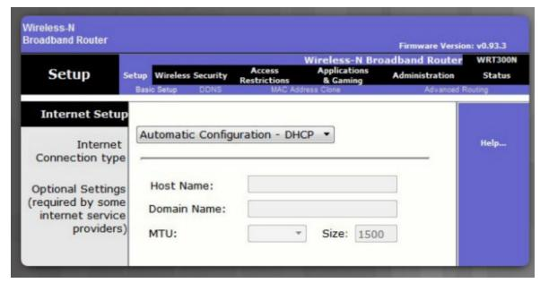
Wireless routers are set to receive IPv4 addressing information automatically from the ISP.
