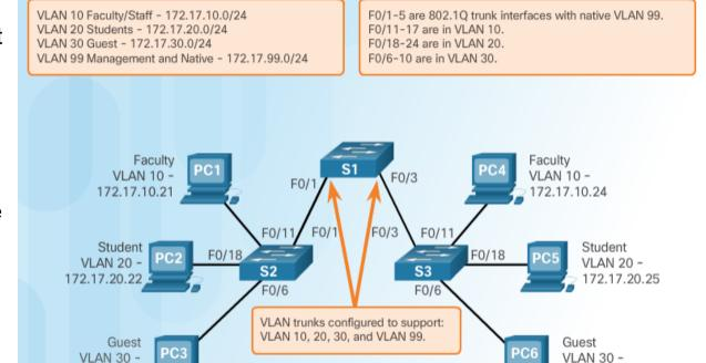
The links between switches S1 and S2, and S1 and S3 are configured to transmit traffic coming from VLANs 10, 20, 30, and 99 across the network.
