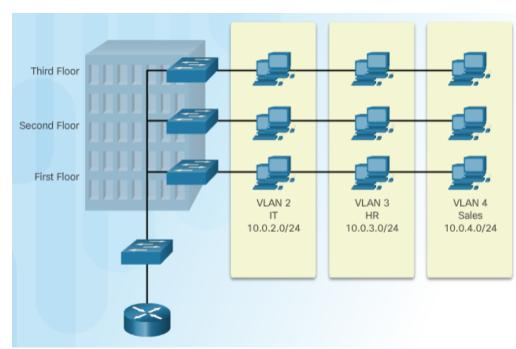
VLANs are mutually isolated and <u>packets</u> can only pass between VLANs via a router.
