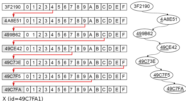
Figure: An example of inserting/searching an object X with an identifier 49C7FA1 into a Pastry network (starting at the node 3F2190).
