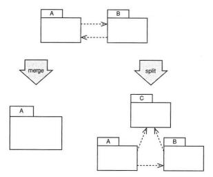
**Component diagram** models a hierarchical decomposition of system into separate parts and the communication relationships between them. It depicts a system's architecture.
