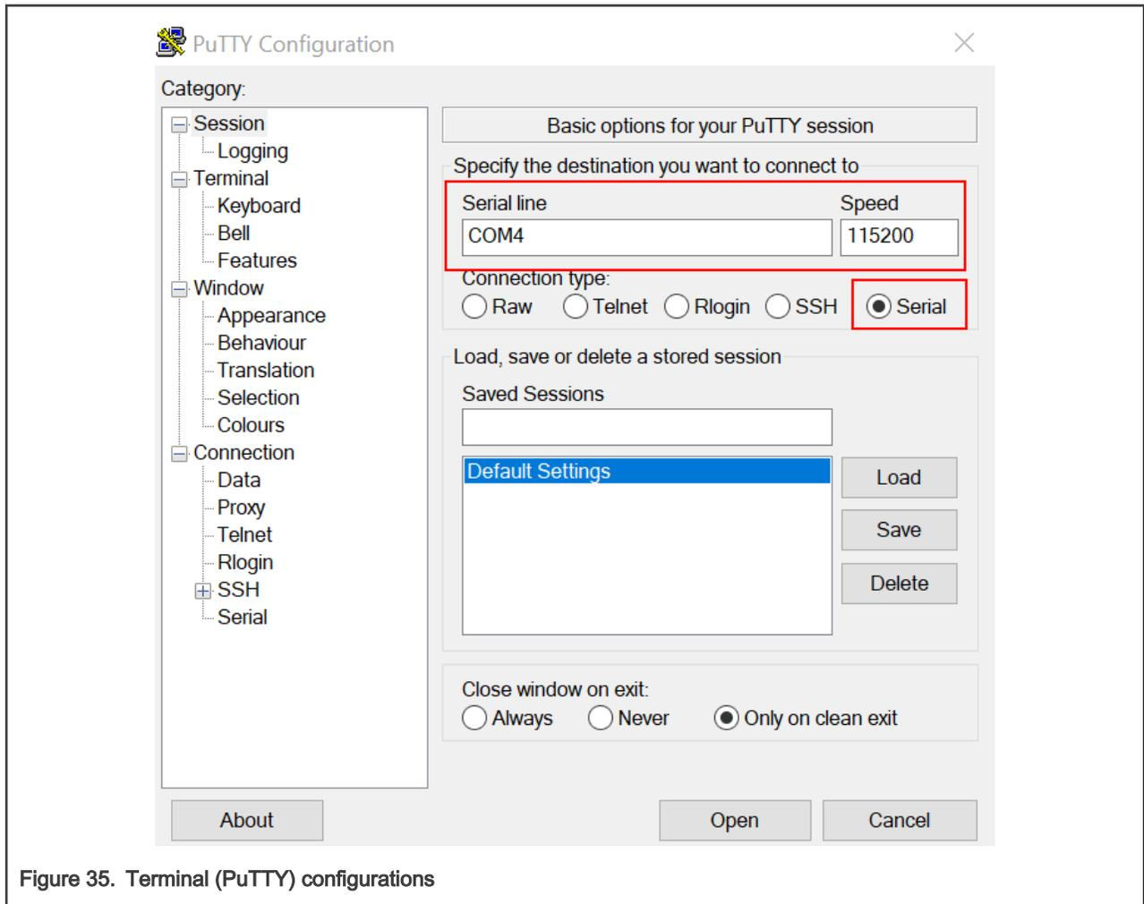
Figure 35. Terminal (PuTTY) configurations
