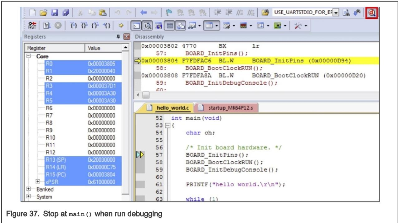
Figure 37. Stop at `main()` when run debugging
