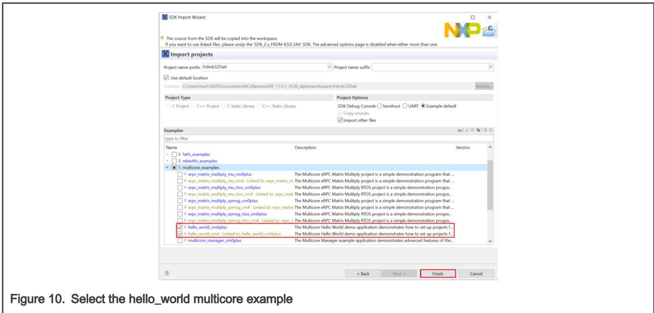
Figure 10. Select the `hello_world` multicore example
