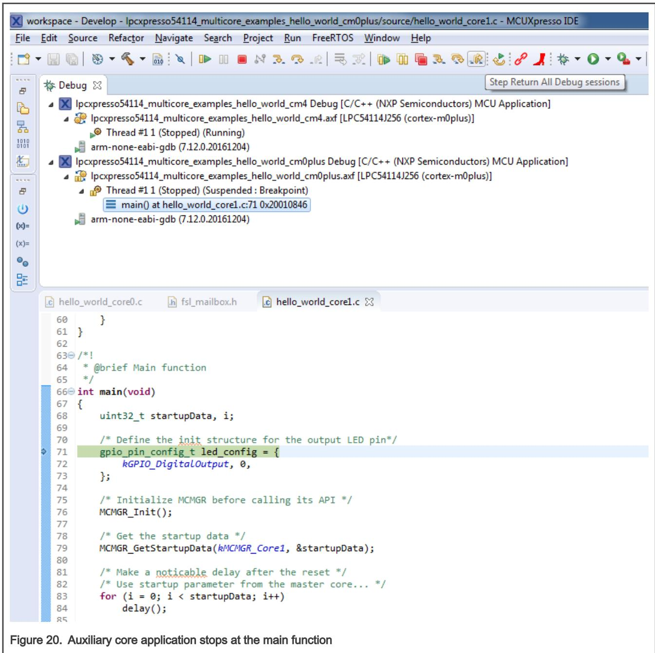
Figure 20. Auxilliary core application stops at the main function
