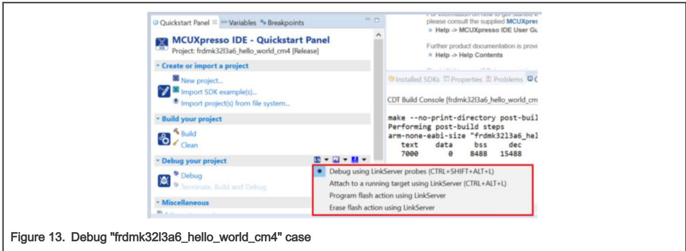
Figure 13. Debug "frdmk32i3a6\_hello\_world\_cm4" case
