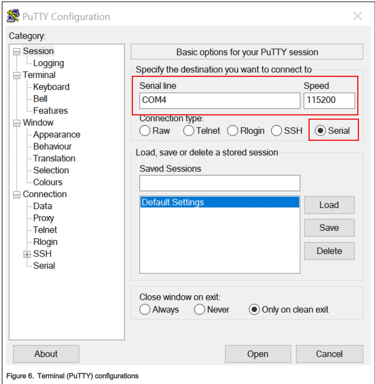
Figure 6. Terminal (PuTTY) configurations
