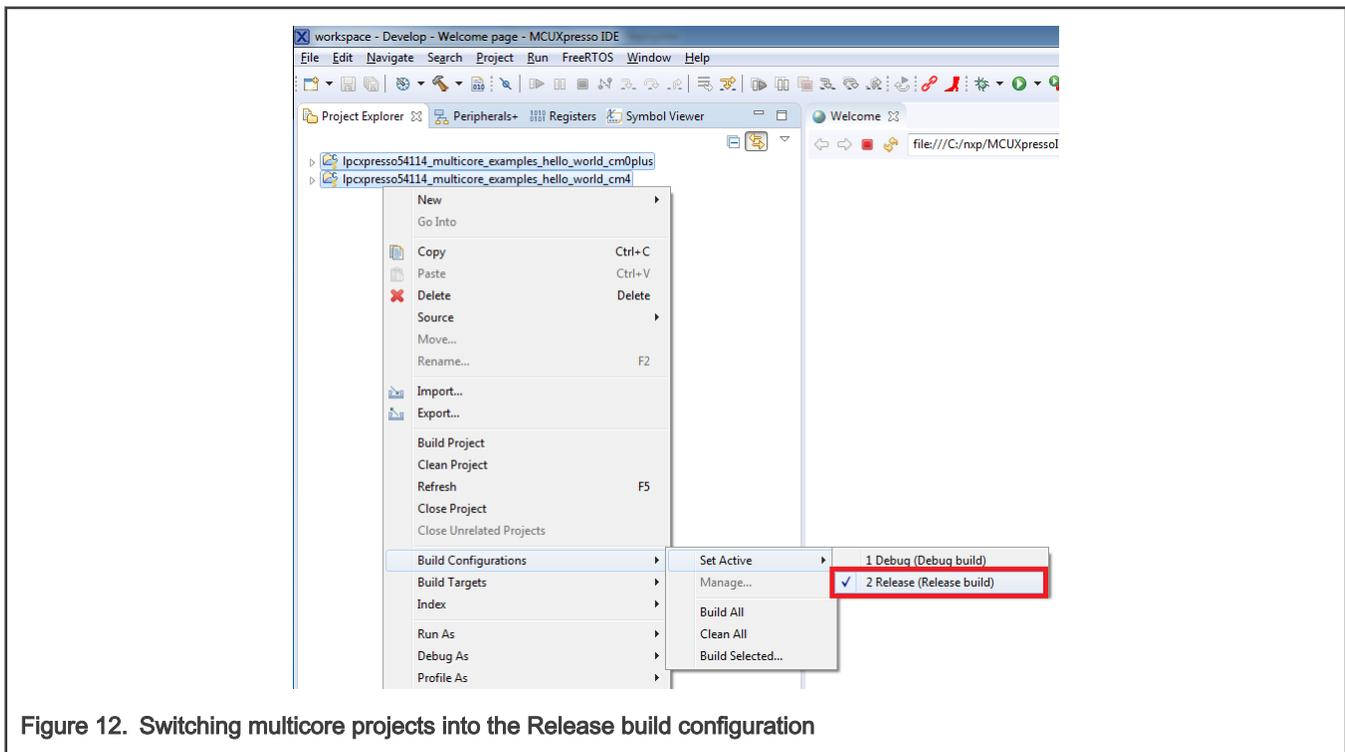
Figure 12. Switching multicore projects into the Release build configuration
