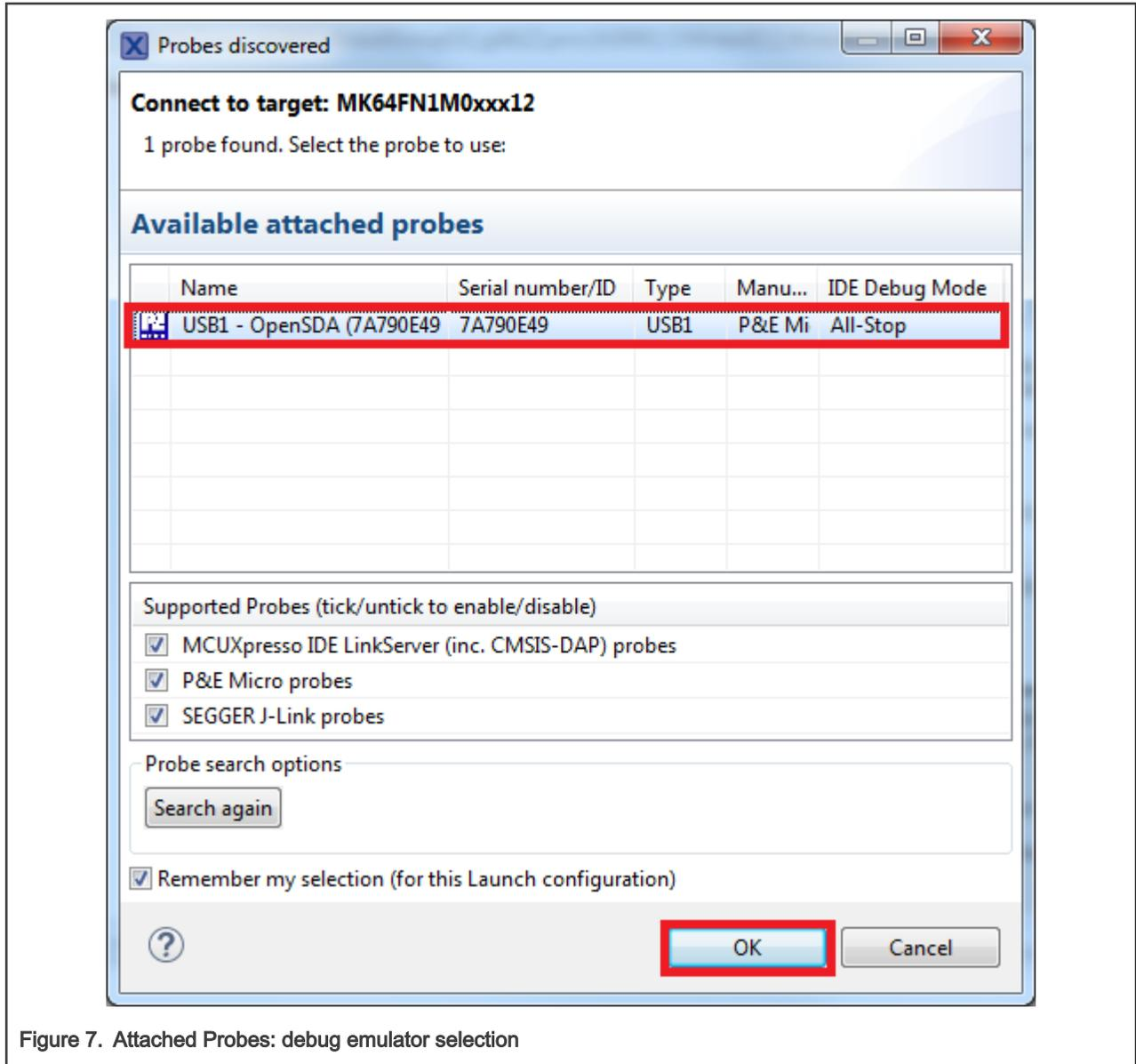
Figure 7. Attached Probes: debug emulator selection
