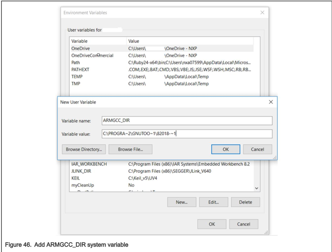
Figure 46. Add ARMGCC\_DIR system variable
