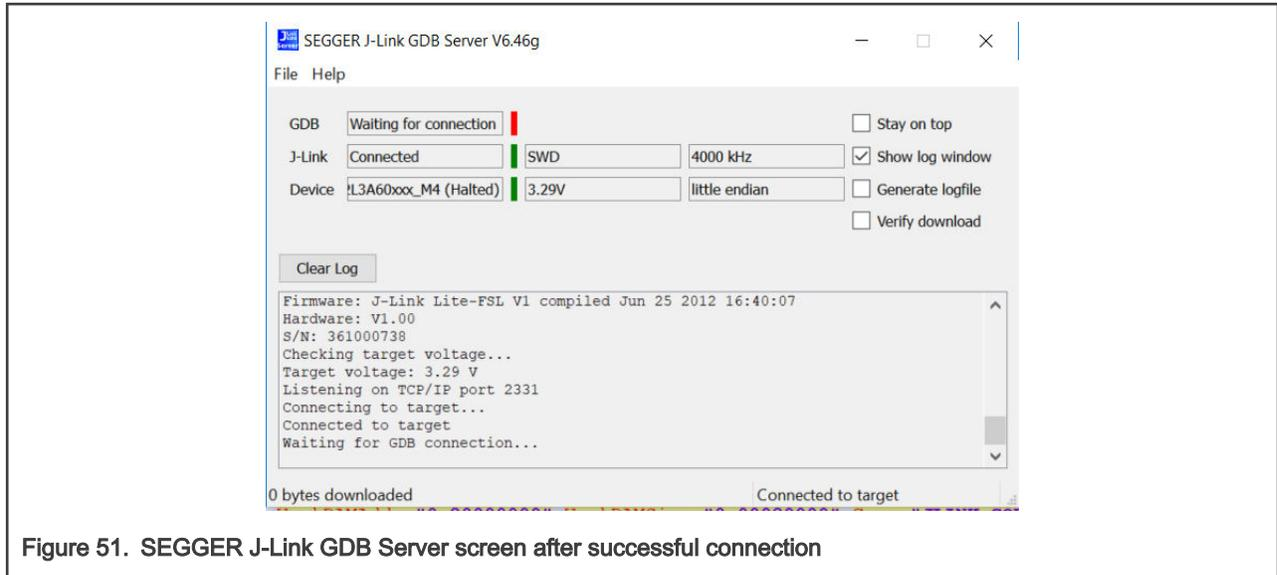
Figure 51. SEGGER J-Link GDB Server screen after successful connection
