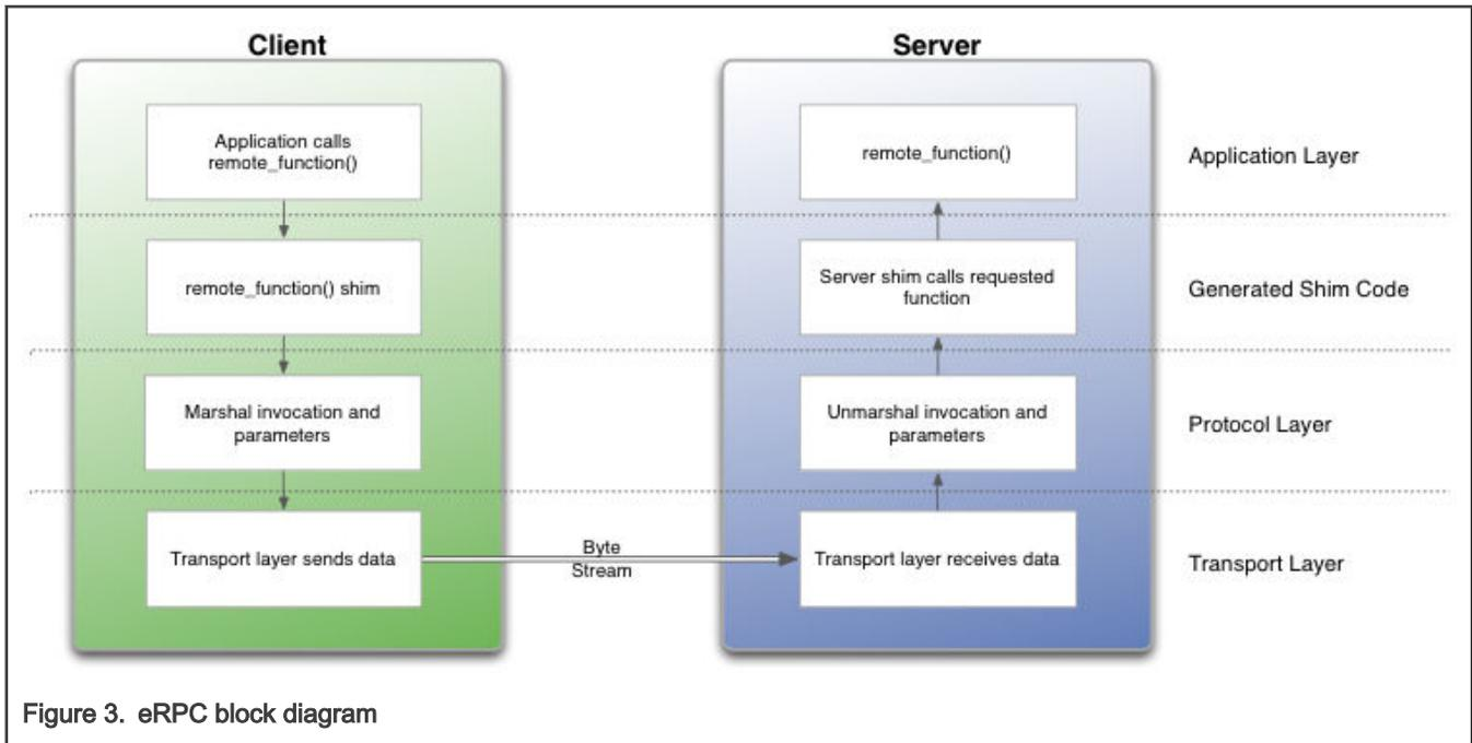
Figure 3. eRPC block diagram
