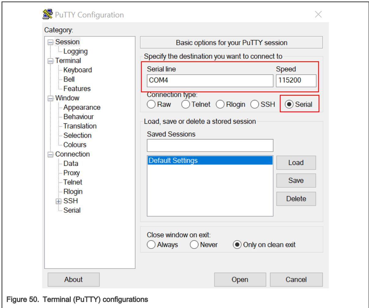
Figure 50. Terminal (PuTTY) configurations
