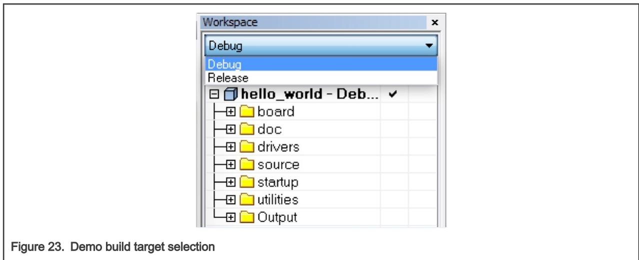
Figure 23. Demo build target selection
