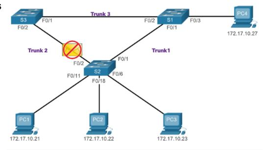
S2 drops the frame because it received it on a blocked port.
