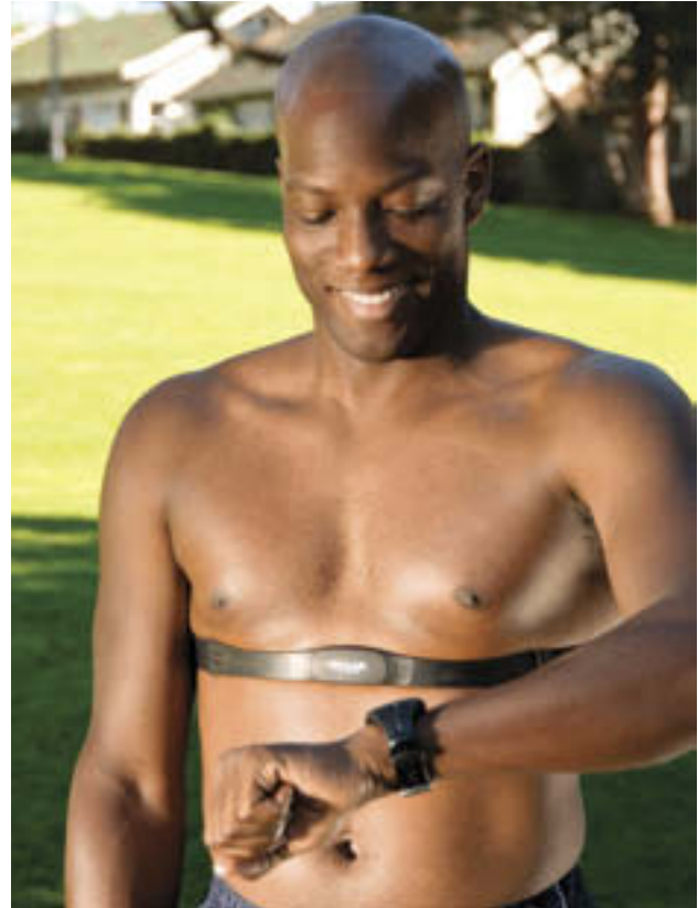
FIGURE 9.5 A runner outfitted with a heart rate monitor. The receiving unit, attached to the chest strap, picks up and transmits electrical impulses from the heart to the digital monitor and memory device worn on the wrist. After the workout, the contents of the memory device can be downloaded to a computer.
