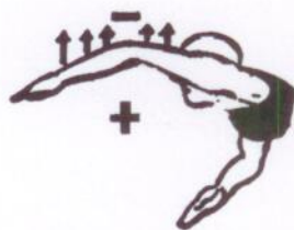
Figure 4.13 Different flow velocities over the upper and lower arm produce a pressure differential.
