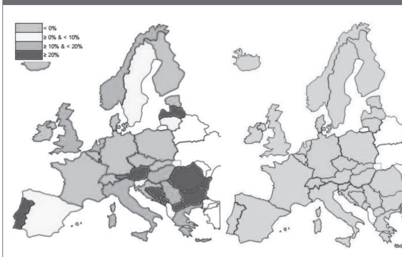
Fig. 44: Generation adequacy per ENTSO-E member country/Regional analysis of generation adequacy; both in January 2025, Scenario B
