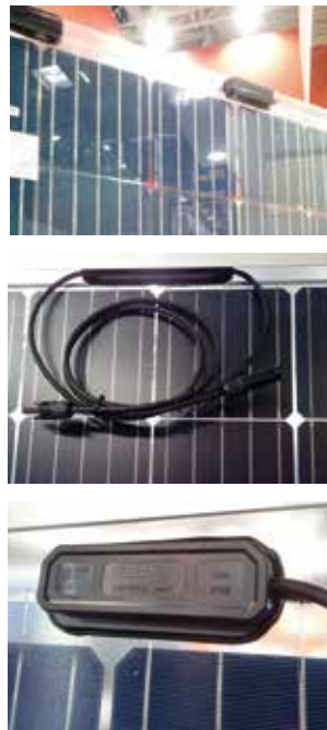
Figure 14 - Bifacial PV modules with a suboptimal design presented at the Intersolar exhibition in 2019 and 2019 (left): the junction box/boxes or the frame shades a part of the backside of the bifacial cells. Other products' design was optimized to prevent shading situations (right).
