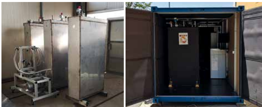
Figure 23 a and b - Modular storage system manufactured (left) and final installation in Container (right)
