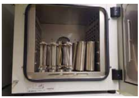
Figure 37 - Holder for several novel polymer liner material to be tested for durability in a test chamber (Source: JKU Linz)
