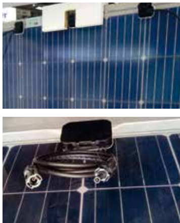
Figure 14 - Bifacial PV modules with a suboptimal design presented at the Intersolar exhibition in 2019 and 2019 (left): the junction box/boxes or the frame shades a part of the backside of the bifacial cells. Other products' design was optimized to prevent shading situations (right).
