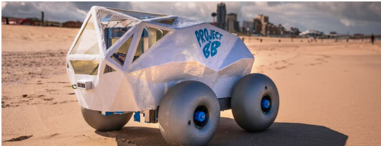
BeachBot uses AI to spot cigarette butts, pluck them out, and dispose of them in a safe bin.
