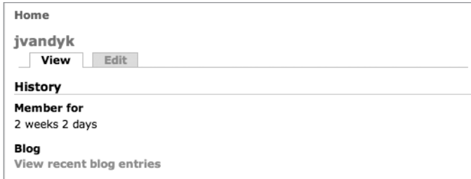
Figure 6-1. The user profile page, with the blog module and the user module implementing hook_user('view') to add additional information
