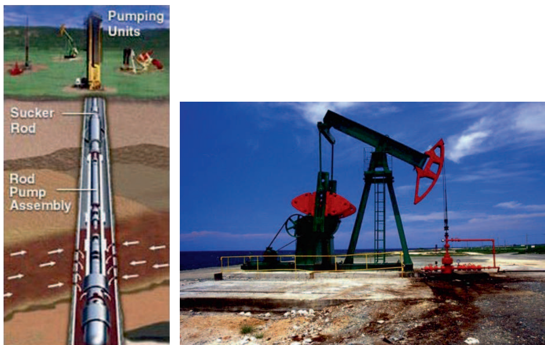
Fig. 8.9. Sucker rod type artificial lift pump for oil production (Printed with permission from [6]).
