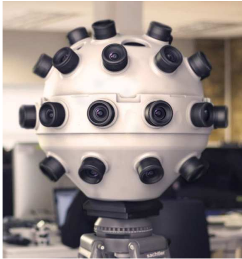
Figure 7.25: The Pantopticon prototype from Figure Digital uses dozens of cameras to improve the ability to approximate more viewpoints so that stereo viewing and parallax from position changes can be simulated.
