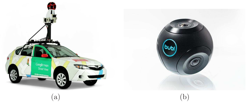
Figure 1.8: An important component for achieving telepresence is to capture a panoramic view: (a) A car with cameras and depth sensors on top, used by Google to make Street View. (b) Bublcam is a cheap, portable way to capture and stream omnidirectional videos.
