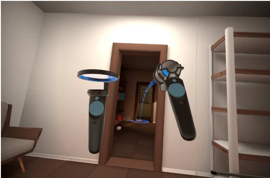
Figure 10.9: A virtual “laser pointer” that follows a parabolic arc so that a destination for teleportation can be easily specified as a point on the floor. (Image from the Budget Cuts game on the HTC Vive VR platform.)
