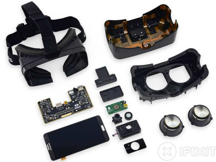
Figure 2.12: Disassembly of the Oculus Rift DK2 headset (image by ifixit).
