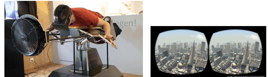
Figure 1.1: In the Birdly experience from the Zurich University of the Arts, the user, wearing a VR headset, flaps his wings while flying over virtual San Francisco, while a motion platform and fan provide additional sensory stimulation. The figure on the right shows the stimulus presented to each eye.
