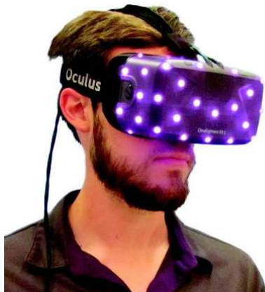
Figure 9.13: The Oculus Rift DK2 headset contained IR LEDs hidden behind IR-transparent plastic. (Photo by Paul Dempsey.)
