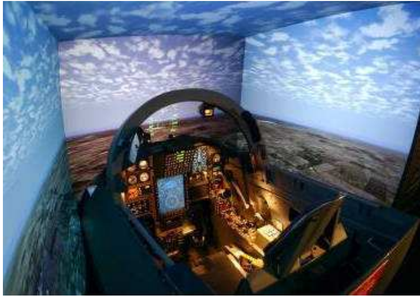
Figure 1.15: A flight simulator used by the US Air Force (photo by Javier Garcia). The user sits in a physical cockpit while being surrounded by displays that show the environment.
