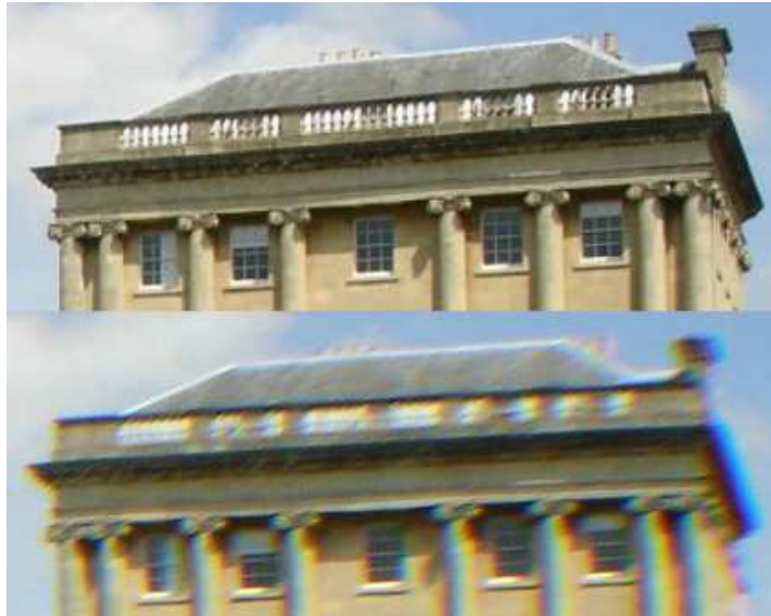
Figure 4.18: The upper image is properly focused whereas the lower image suffers from chromatic aberration. (Figure by Stan Zurek.)
