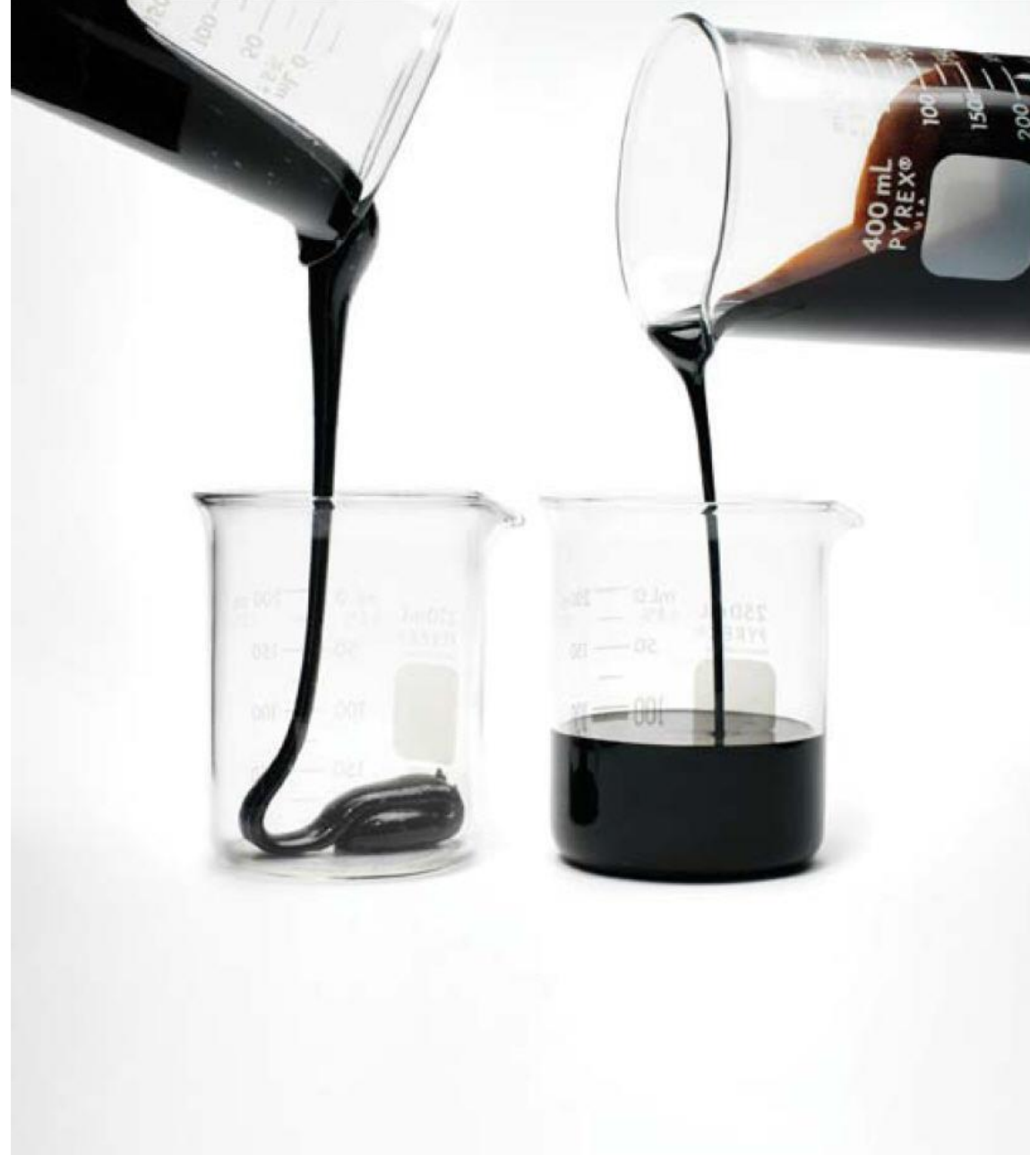
Alberta's crude oil (left) feels and flows like asphalt or molasses. (Courtesy of: Petrobank Resources).
