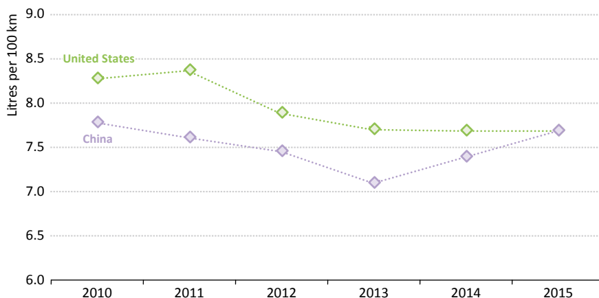
Figure 3.5 ▶ Fuel economy of new passenger car sales in the United States and China
