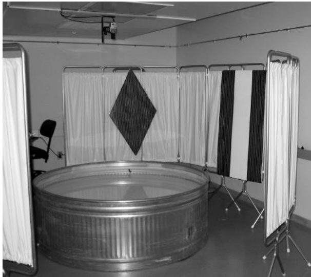
FIGURE 2.7 The Morris water maze is one of the most common rodent tests for learning and memory. Courtesy of the Stanford Behavioral and Functional Neuroscience Laboratory.
