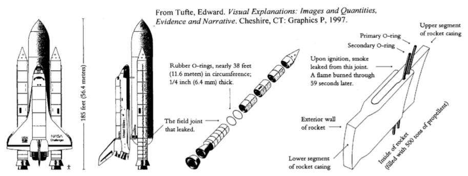
The shuttle consists of an *orbiter* (which carries the crew and has powerful engines in the back), a large liquid-fuel *tank* for the orbiter engines, and 2 solid-fuel *booster rockets* mounted on the sides of the central tank. Segments of the booster rockets are shipped to the launch site, where
