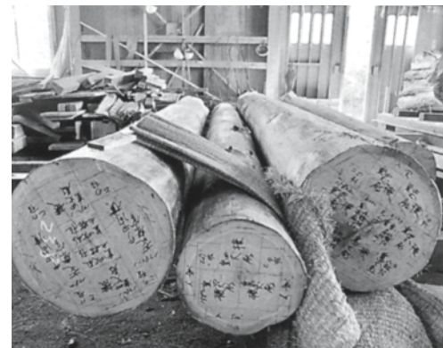
Fig. 55: Three tree trunks marked ready for cutting in the sawmill Visible here are the marked-out sections plus additional information such as building name, component name, component number, and trunk number.
