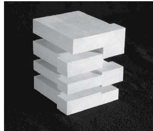
Fig. 40: Wooden model Shows the different ceiling heights and how the apartments are "stacked".
