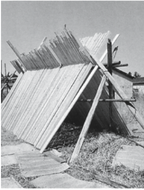
Fig. 56: Boards stacked for weathering
