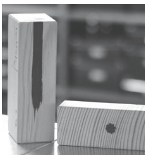
Fig. 37: Wood welding The application of ultrasonic energy causes the plastic to form a connection with the wood at the macroporous level.
