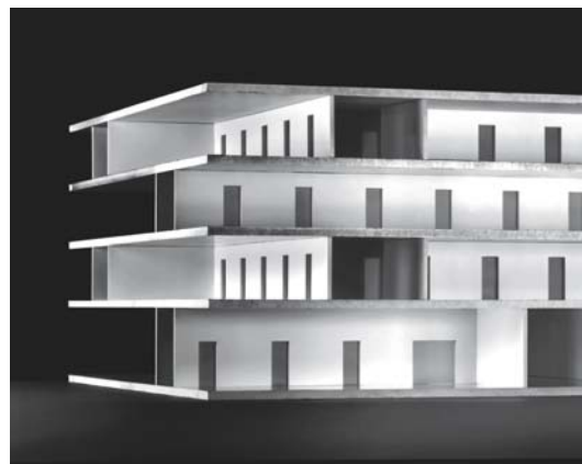
Abb. 64: Model of loadbearing structure with shear walls offset or rotated through 90°
