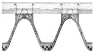
Fig. 8: Detail of floor construction: V-shaped precast ferro-cement elements; wall thickness: 3 cm; total depth of floor (incl. floor finish): 50 cm Pier Luigi Nervi: Galbani office building, Milan (I), 1955/56
