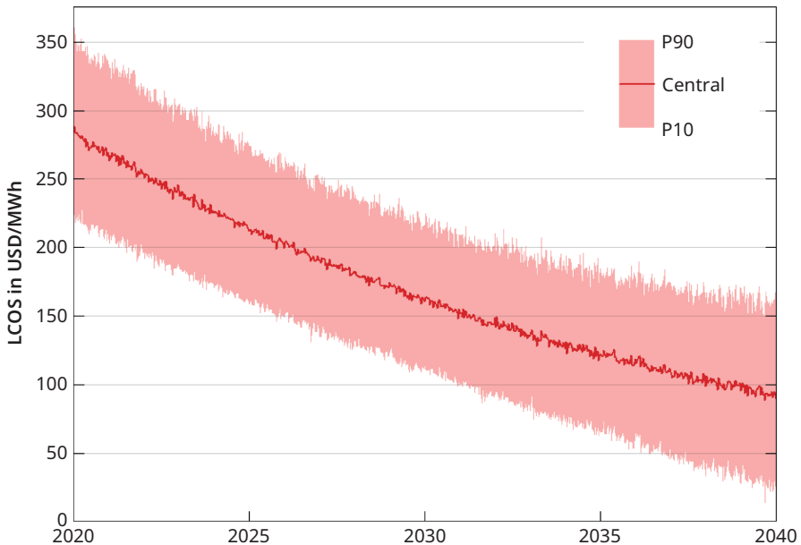
Figure 5.6 Reduction of lifetime cost (levelized cost of storage in USD/MWh) from 2020 to 2040 based on the 2020 input parameters in Table 5.1 and the relative change to these parameters given in Table 5.3. The 10th and 90th percentiles are based on the uncertainty and uncertainty increase indicated in Table 5.3. Chart from < www.EnergyStorage.ninja >.
