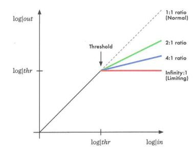
The gain computer is the part of the compressor that generates the control voltage (CV) and calculates the amount of compression applied to an audio signal. Once the input signal exceeds the threshold point, it is attenuated according to the ratio setting. Ratios of 2:1 to 8:1 are generally considered normal compression, while ratios of 10:1 or higher are called limiting.
