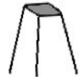
Too Steep-Trans Am Building (not rigid-vibrations)
