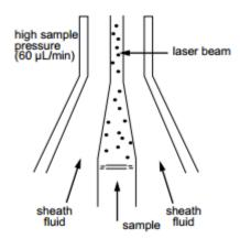
particles pass through the laser intercept, they scatter laser light. Any fluorescent molecules present on the particle fluoresce. The scattered and fluorescent light is collected by appropriately positioned I\_\_\_\_s. A combination of beam splitters and filters brings the scattered and fluorescent light to the appropriate detectors. The detectors produce electronic signals. These signals correspond with the optical signals striking the detectors.
