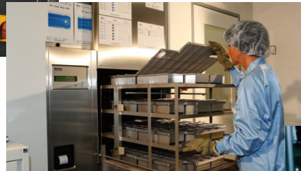
Cleaned endodontic instruments are transported through a double door system into the clean room
