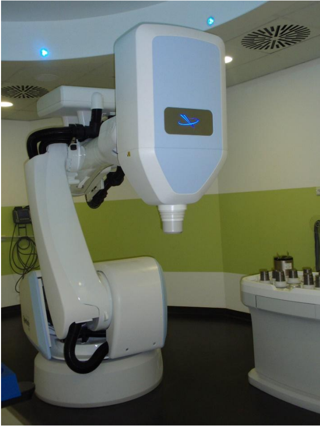
Fig. 6: CyberKnife - a robotic irradiator
