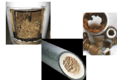
Hardness minerals precipitate out of the water and form energy robbing scale.
