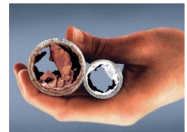
Hardness minerals precipitate out of the water and form energy robbing scale.
