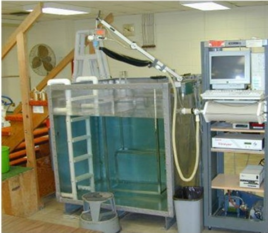
Hydrodensitometer. Courtesy of Human Performance Lab, University of Wisconsin-La Crosse.
