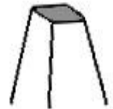
Too Steep-Trans Am Building (not rigid-vibrations)
