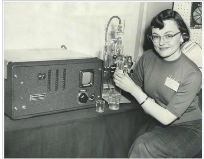
Figure 5.4. The first trade-show exhibition of the Model A counter. [207] According to the Sun-Times legend, Ms. "Virginia Mackay of the University of Chicago demonstrates a Coulter automatic blood cell counter and cell-size analyzer at Conrad Hilton Hotel."
