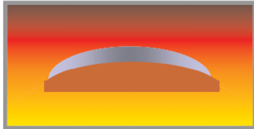
b) Slumping a glass blank (forming)
