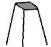
Too Steep-Trans Am Building (not rigid-vibrations)
