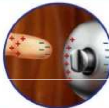
C Charging by Induction The negative charge on the girl's fingertip produces an electric field that repels the electrons and attracts the protons on the doorknob. An area of positive charge is induced on the edge of the doorknob just by coming near (without touching it). If another person touched the doorknob's negative side, the electrons would be transferred away from the doorknob, leaving it with an overall positive charge.
