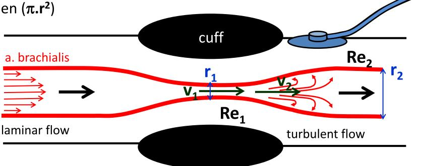
closely behind narrowing of the artery:  $S_1 < S_2$  a  $v_1 \approx v_2 \rightarrow Re_1 < Re_2 \rightarrow$  turbulent flow
