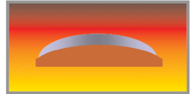
b) Slumping a glass blank (forming)
