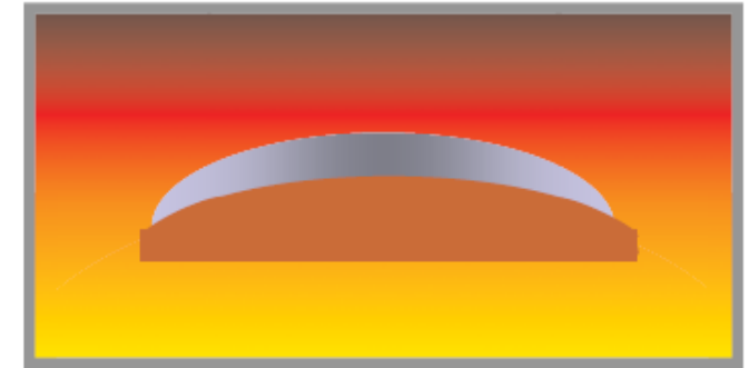
b) Slumping a glass blank (forming)
