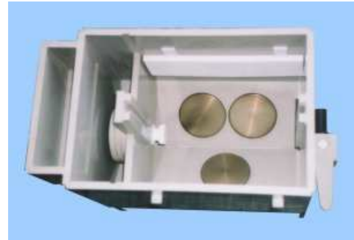
ultrasonic bath seen from above (circular plates are sources of ultrasound)
