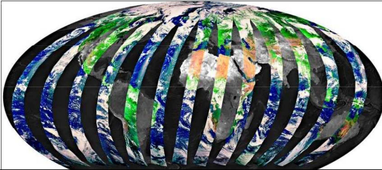
7. Sun synchronous Envisat ground track during one day and coverage of geostationary Meteosat (at 0 degree longitude).
