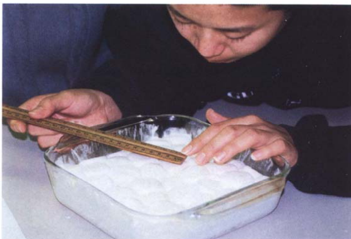
Physics student Mia Youhne measures the distance between melted spots and calculates the speed of light. (Photo by Ashley Miller.)
