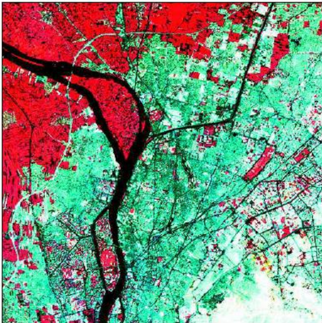
4. Combination of Landsat ETM bands 4,2,1 to form an infrared false colour satellite image of Cairo
