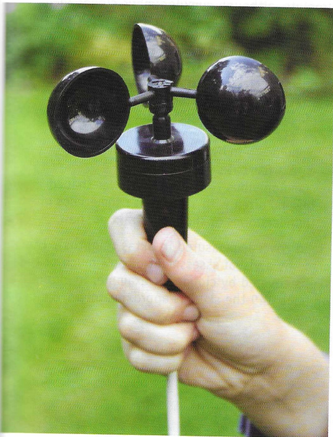
▲ Figure 2.91 An anemometer
