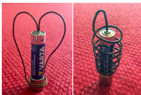
A battery and a copper wire are used to demonstrate the Lorentz force.
