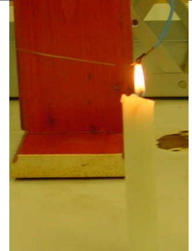
Thermocouple (Candle instead of concentrated sunlight)
