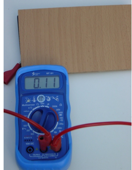
darkened: U = 0,11 V (Infrared radiation)
