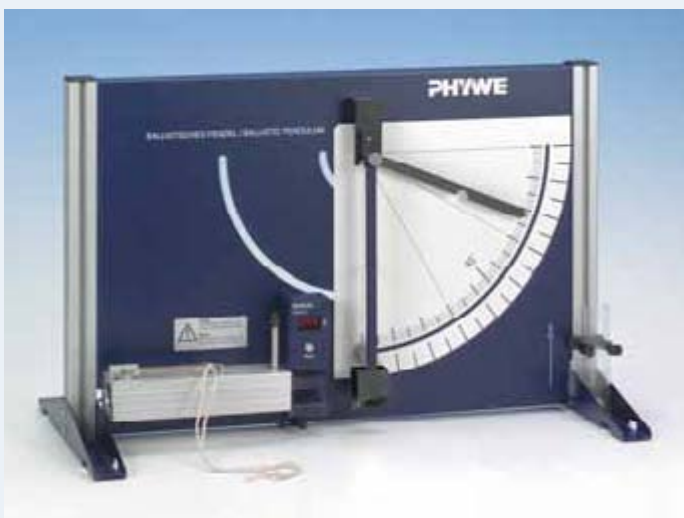
Experimental set-up with supplement for direct measurement of the initial velocity of the ball.
