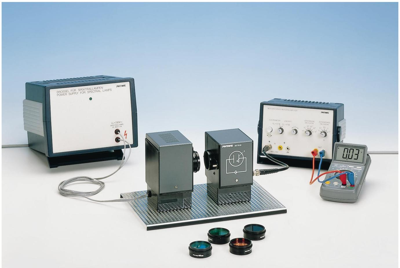
If a photon of frequency  $f$  strikes the cathode, then an electron can be ejected from the metal (external photoelectric effect) if there is sufficient energy.
