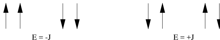
Figure 15.1: The interaction energy between nearest neighbor spins in the absence of an external magnetic field.
