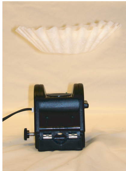
Figure 3.2: A falling coffee filter does not fall with constant acceleration due to the effects of air resistance. The motion sensor below the filter is connected to a computer which records position data and stores it in a text file.
